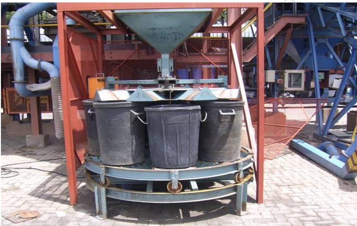
Figure 3.1 Rotary bulk splitter used to split ten-ton bulk sample.
