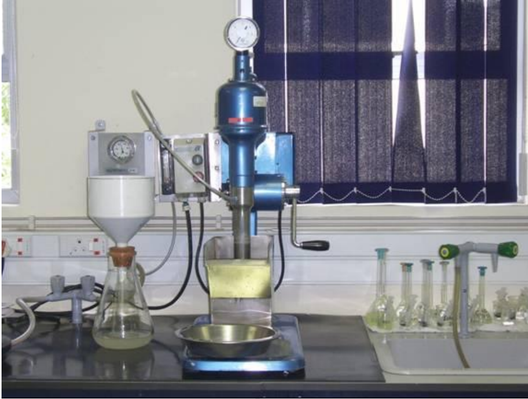
Figure 3.5 Denver flotation cell used for laboratory batch flotation tests.
