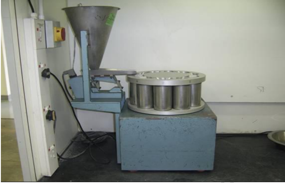
Figure 3.2 Rotary splitter used to split 5 kg sample to 500 g portions.
