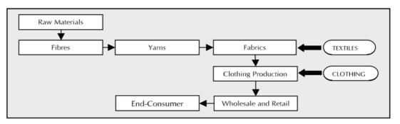
Fig. 1 The Simplified Clothing -Textile Pipeline
